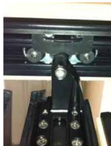
Photo 20 Completed stacking catch
