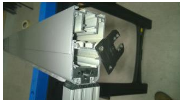
Photo 6 Side jamb connected to top track
