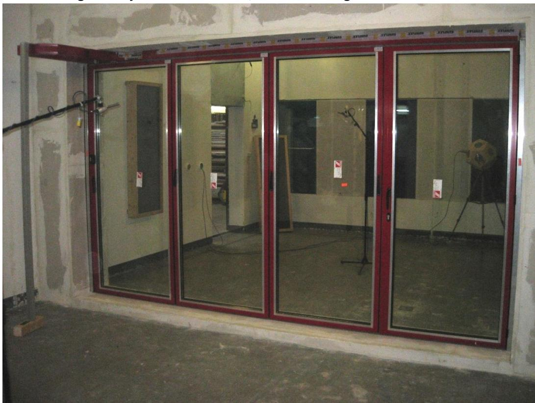
**Fig. 4: Horizontal-Sliding-Wall-System SF 50 H-S-W, View Receiving Room, Detail connection below**
