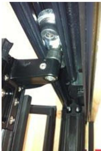
*Photo 17 – adjustment bolt with collar*
