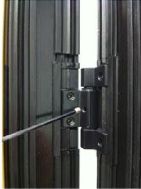
*Photo 11 – Securing hinge pins*
